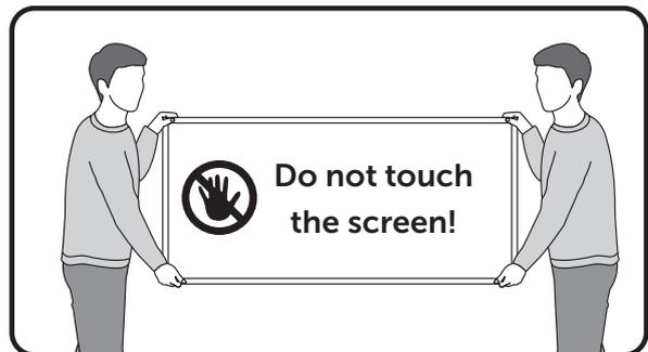
There is a risk of damage to the screen if it is handled incorrectly. We recommend lifting the TV by holding it by the edges, as shown in the picture.
